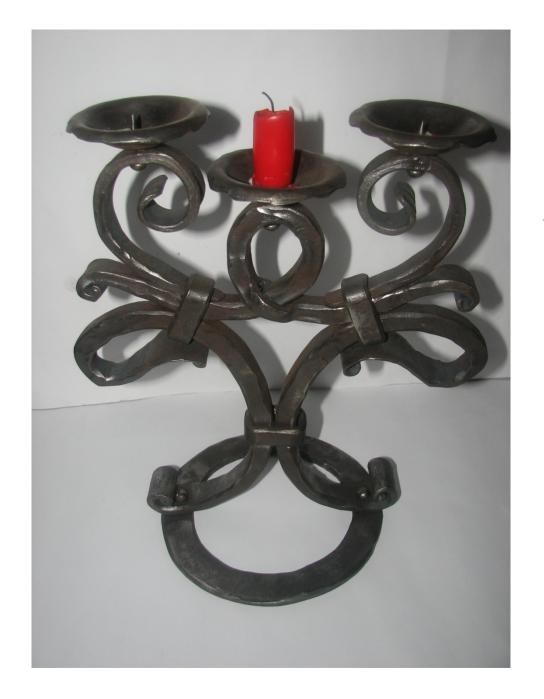
It is also a very hard job because one has to heat the iron and shape it by hand with a hammer.
